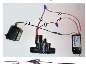
self-adhering tape making sure to create a proper watertight seal. Plug the power supply connector into the black sensor power connector and seal with self-adhering tape. Apply a liquid electrical sealant (available at most hardware stores) to each connection. We recommend that the unit be tested before weatherproofing the connectors.
