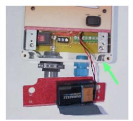
Install the battery provided into the battery housing and attach connector. Replace access cover. Mount controller on wall using the #6 screws provided in the four holes in corner indicated by the green arrow (Left) (do not make holes in controller housing!). Or mount on the optional pole mount using the hardware provided.
