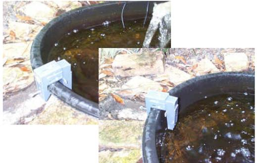
*Note: The spillway may be mounted directly to the side of the pond using the two screw holes on either side in back by removing the slide mount. If your pond requires a different mount, please contact Aquility Systems for a replacement.*
